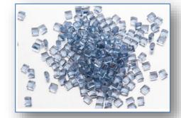
Fluoropolymer resins are used to manufacture products, where heat, low coefficient of friction or chemical resistance are needed
